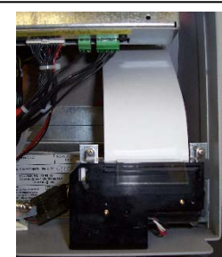
Figure 3: Feeding paper Insert paper into feeder – wait 2 seconds until it catches onto feeder
