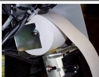
Figure 2: Pin & Paper Remove pin, insert pin into new paper roll, lay pin and paper roll back onto frame. Paper feeds from the top of the roll.
